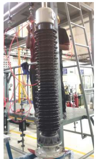
Porcelain part replacement, bushing refurbished and supplied after complete routine testing
