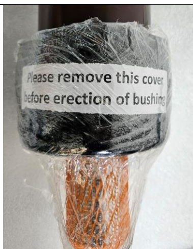
Figure 7 : Electrode With PVC cap protection
