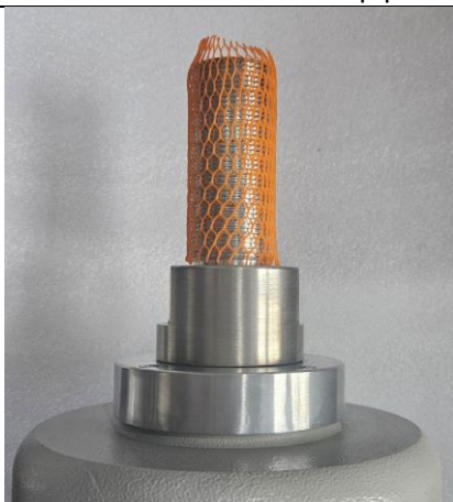
Figure 8 : Terminal Protection with PVC mesh
