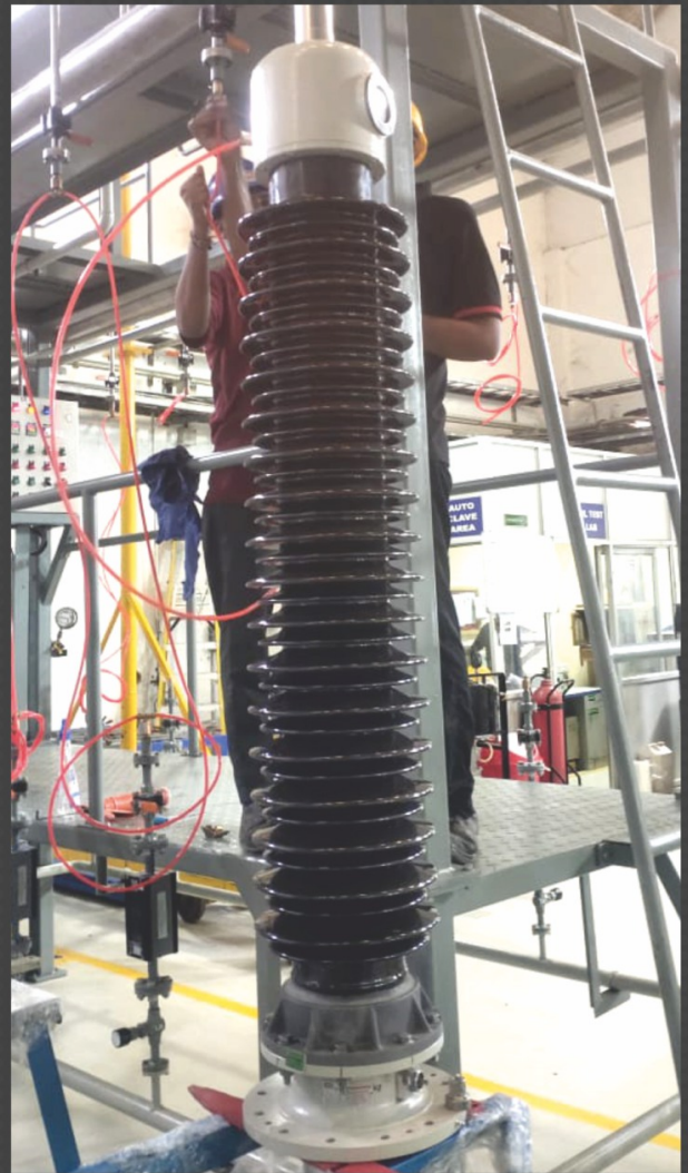
Porcelain part replacement, Bushing refurbished and supplied after complete routine testing
