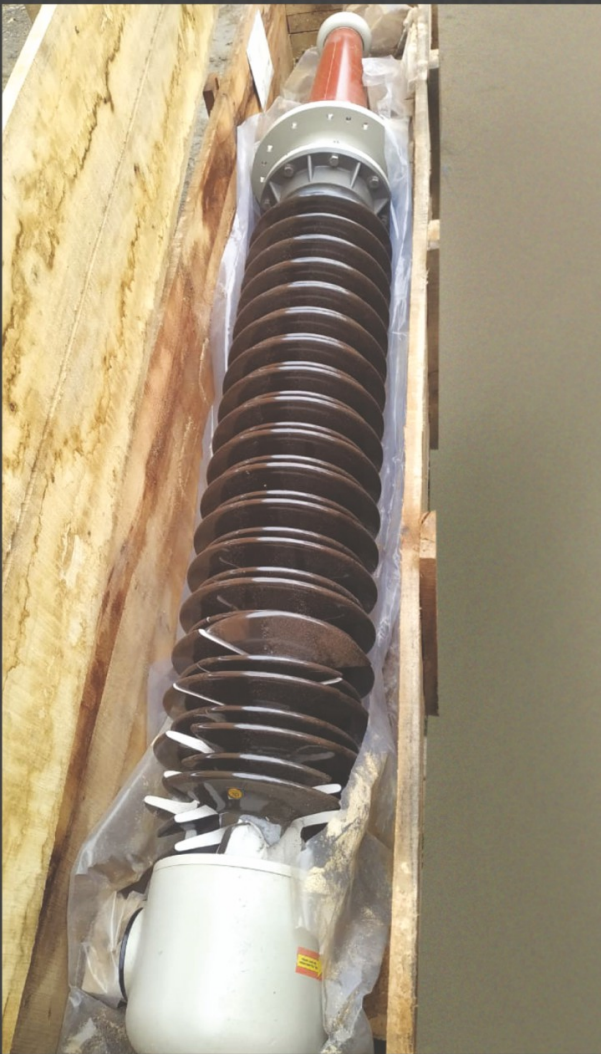
145 kV OIP bushing with transit damage to Air end porcelain
